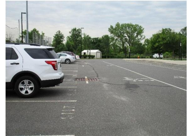
The high school is new with internal drainage. Parking spaces can be replaced with pervious pavement to capture and infiltrate stormwater. Rain gardens can also capture, treat, and infiltrate runoff. A preliminary soil assessment suggests that more soil testing would be required before determining the soil's suitability for green infrastructure.
