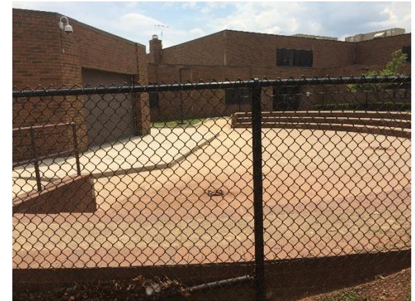
A bioretention system can be installed on the northeast side of the school to capture, treat, and infiltrate rooftop runoff. The outdoor concrete stage base, and a row of parking spaces, can also be replaced with pervious pavement to capture and infiltrate stormwater. A preliminary soil assessment suggests that more soil testing would be required before determining the soil's suitability for green infrastructure.
